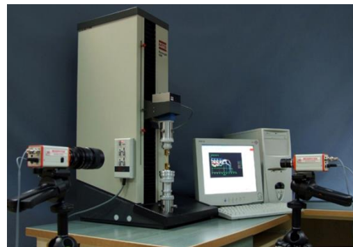
Figure 1: Experimental set-up; testing machine Synergie 100 (MTS) and videoextensometer (ME 46-350, Messphysik) [2].
